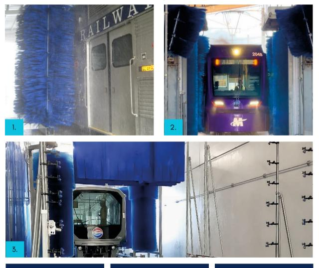
vertical brushes ideal for cleaning flat surfaces and square corners eaves brushes supplement vertical brush cleaning for rounded or nonsquare corners
