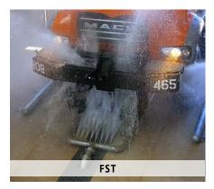
The InterClean FST and CTW type Chassis washes are designed specifically to provide enhanced cleaning, salt removal, and demucking of the vehicle's undercarriage using high-volumes of fresh or reclaimed water.
